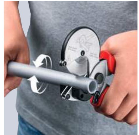
Makes cutting particularly easy: the rotating cutting wheel allows the pipe to be rotated in the pipe cutter with little friction, or, vice versa, the pipe cutter can be rotated around the pipe.
