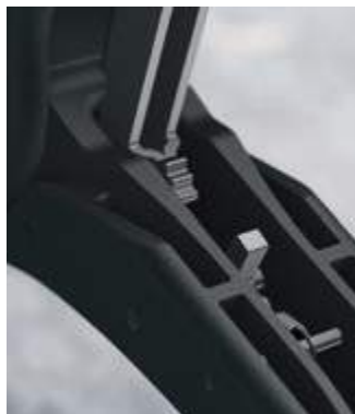
The ratchet crimping mechanism ensures the correct crimping pressure.
