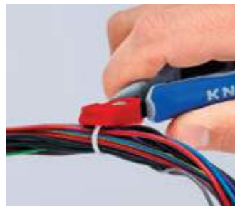
Remove the head of the cable tie using the Electronics Diagonal Cutter...
