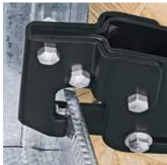
The punching tool is squeezed through the metal section sheets
