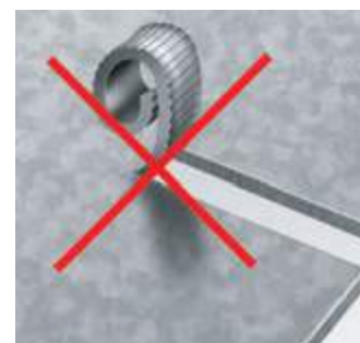
Notching without chip breaking
