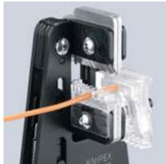
12 12 02 with cable guide and length stop
