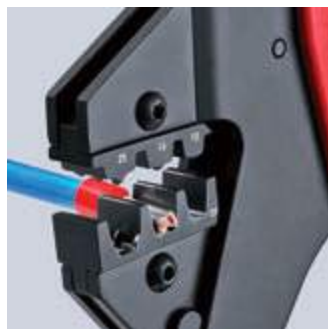
97 43 200 with crimping dies 97 49 09 for wire ferrules
